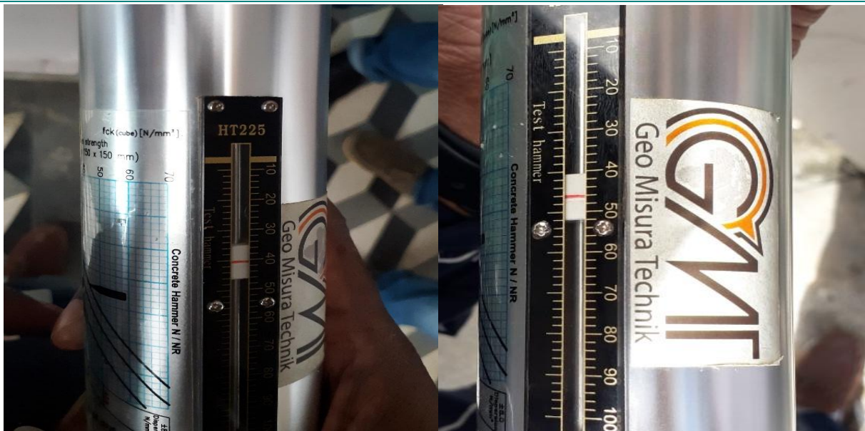
FIGURE 1-12: PHOTO SHOWING REBOUND HAMMER TEST RESULT
